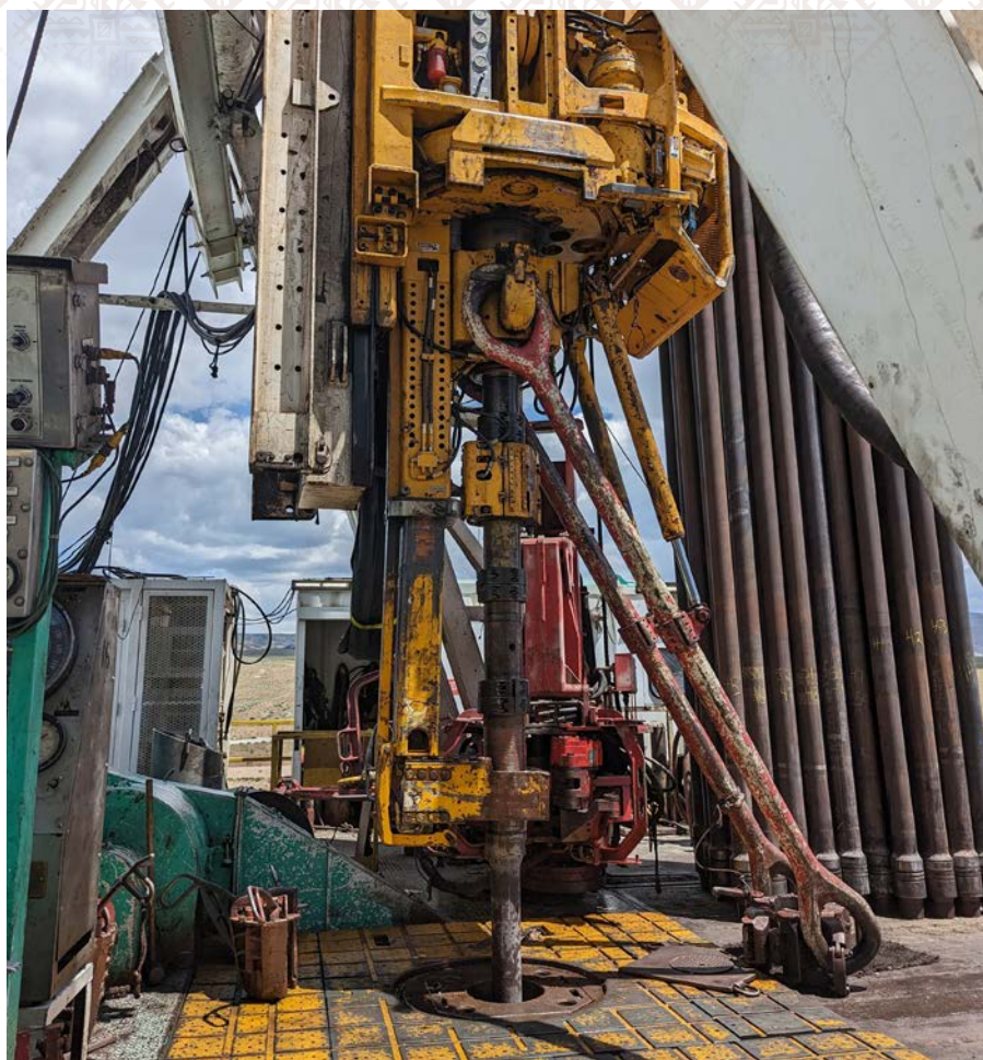
The drill at Utah FORGE, which is currently drilling a 10,000-foot-deep geothermal well to test Enhanced Geothermal Systems.
